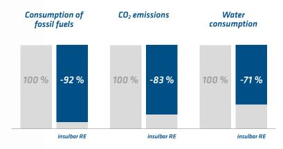
The outstanding ecological balance of insulbar RE is already apparent at the manufacturing stage. Here it is shown in comparison with a conventional insulating profile from non-recycled polyamide.
